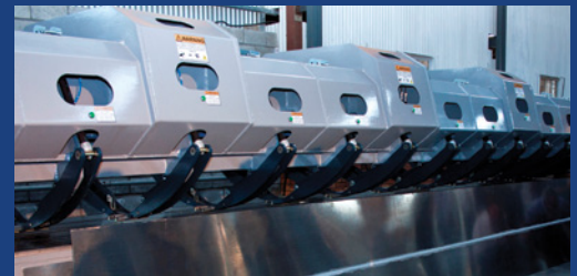
Friction welding platform and 8metre friction stir weld - the longest weld in Africa
